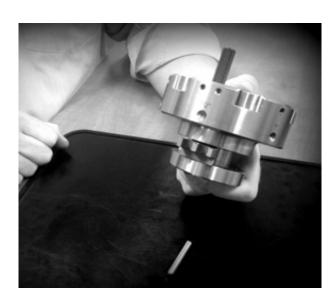
3) Take out the chain guide and replace it by a new chain guide.
