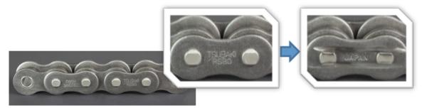
• Quad stake rivet: Apply grinding.
