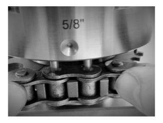
5) Make sure that the pins of the chain breaker are directed at the centre of the chain pins. By using continuous pressure, without shocks, push pins out of the chain by using the lever. Put the lever back into its original position, remove and disassemble the chain.
