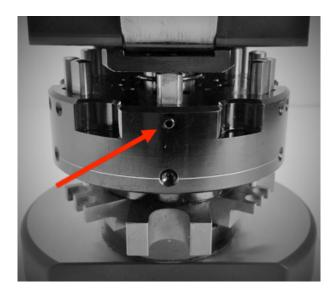
Adjust the screw until you reach a free movement of the cutting pin and at the same time ensure that it cannot be pulled up.
